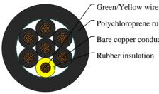
Polychloroprene rubber outer jacket Bare copper conductor Rubber insulation
